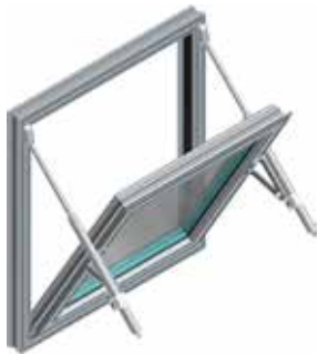
Fig. 52 mcr OSO THERM 75 smoke exhaust window with two S spindle actuators with shifted pivot point
